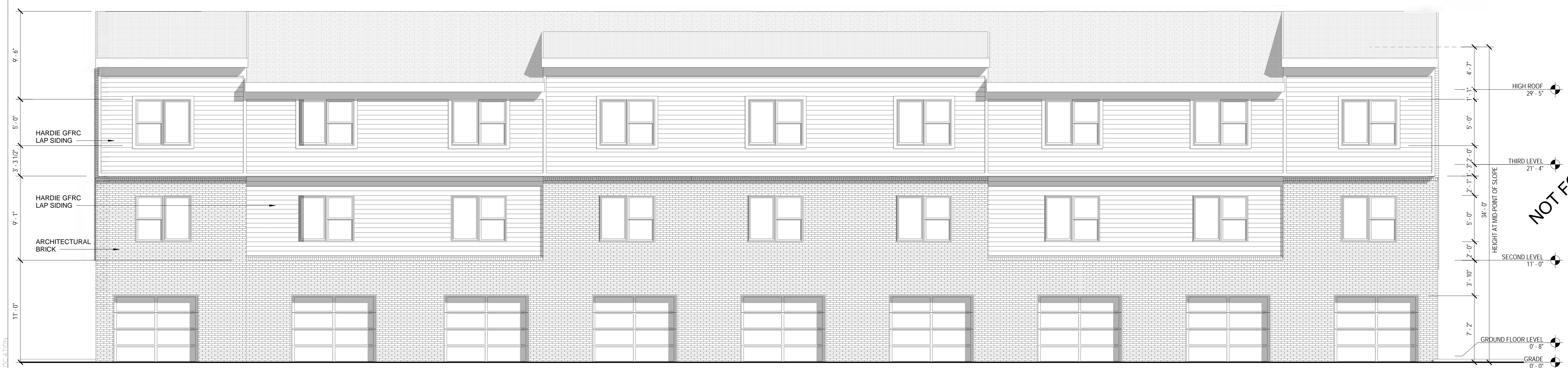
1 NINE-UNIT BUILDING - REAR ELEVATION SCALE: 3/16" = 1'-0"
