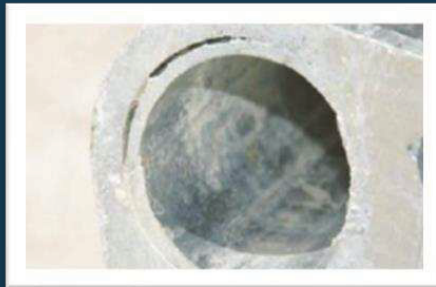
HDG After Fabrication Galvanized Inside and Out 100%
