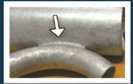
Completely Galvanized at weld point (Hot-Dip Galvanization)
