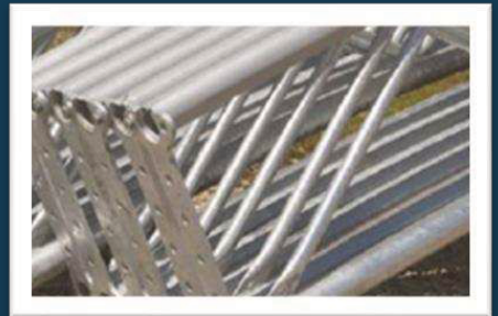
Completed Hot Dip Galvanized Trusses
